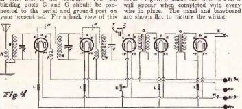
unit look at Figure 3. The A and B batteries of the regular set may be used. The rheestat E should have the proper resistance for the tube used and the variable condenser C is .00035 microfarad capacity
